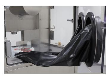
Figure 3: Reinforced seals for nitrogen flooding
